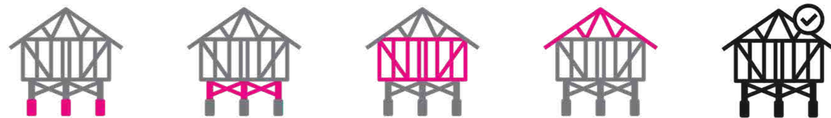
Figure 18: Typical concept of Tie Down from Bottom Up. (Graphics adapted from Kaunitz Yeung Architecture, 2017)
